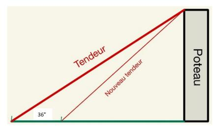
From the turnbuckle anchor point, located 18 meters from the base of the post ("Poteau"), the top of the post can be seen at a 36° angle.
